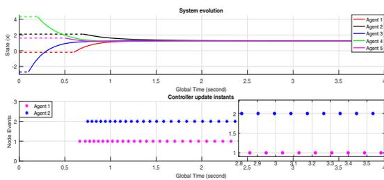
Fig. 3: State trajectories and edge event times both agents 1 and 2 triggered over edge  $\epsilon_1$
